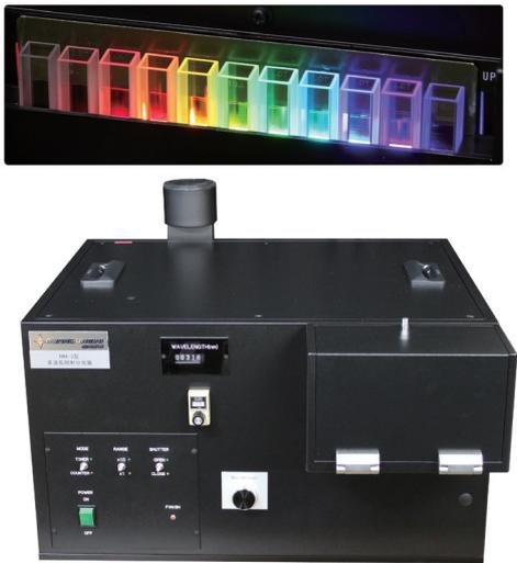
The Model MM-3 is capable of irradiating multiple samples simultaneously ( for example, 11 pcs of rectangular cell 10mm x 10mm ) in each wavelength band of 220-520nm and 400-700nm.
